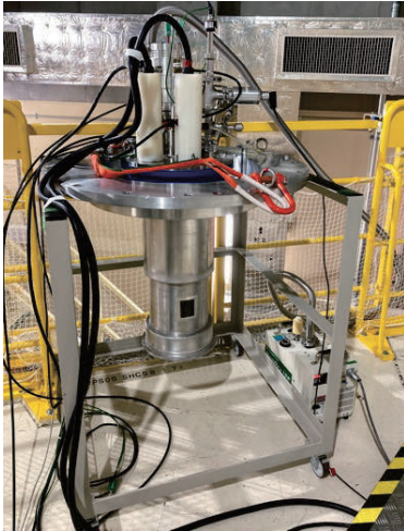
Figure 1: Vanadium high-temperature furnace
