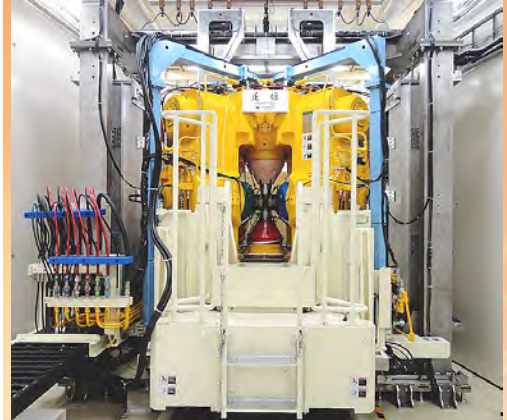
The 6-axis multi-anvil press "ATSUHIME".
