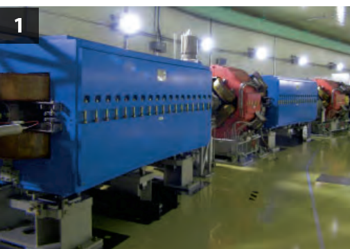
3GeV Proton Synchrotron The proton synchrotron, which comprises the electromagnets to accelerate the protons from the linear accelerator, is arranged in a ring. This synchrotron accelerates protons to 3GeV (about 97% of the speed of light).
