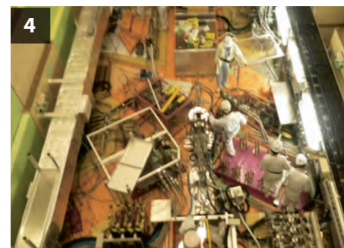
Muon Beam Extraction The 3-GeV proton beam is focused on the muon target located at M2 tunnel, upstream of the neutron target. From the muon target, four muon beam lines, D-line, U-line, S-line and H-line are installed to extract intense pulsed muons.
