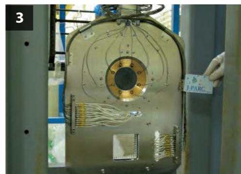
Muon Target The target to produce \pi -mesons which decay to muons. The target, being made up of carbon, is surrounded by a copper radiator for heat generated with proton irradiation.
