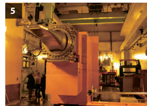
Neutron Target The target truck for producing neutrons. The mercury target cooling system cycles mercury, allowing the heat from the proton collisions to be removed.
