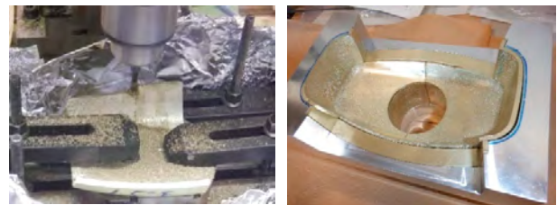
Figure 3. NC milling machine (Left) and upper part of the decoupler (Right).
