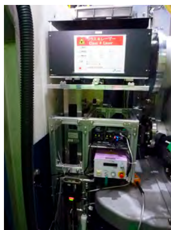
Figure 1. Newly installed setup of the SEOP system. The neutron beam goes directly through the black box (SEOP box), where the glass cell for the ^3\text{He} gas filter is positioned.
