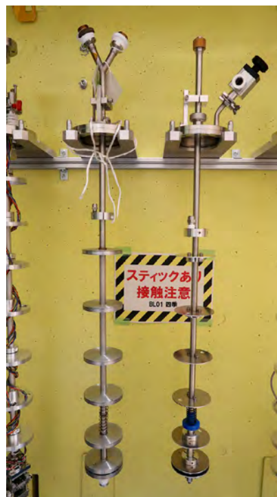
Figure 1. The old (left) and new (right) low-temperature sample sticks.
