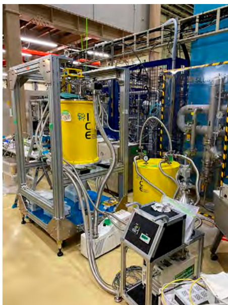
Figure 1. Snapshot of the new cryogen-free variable temperature cryostat placed at the test bench.
