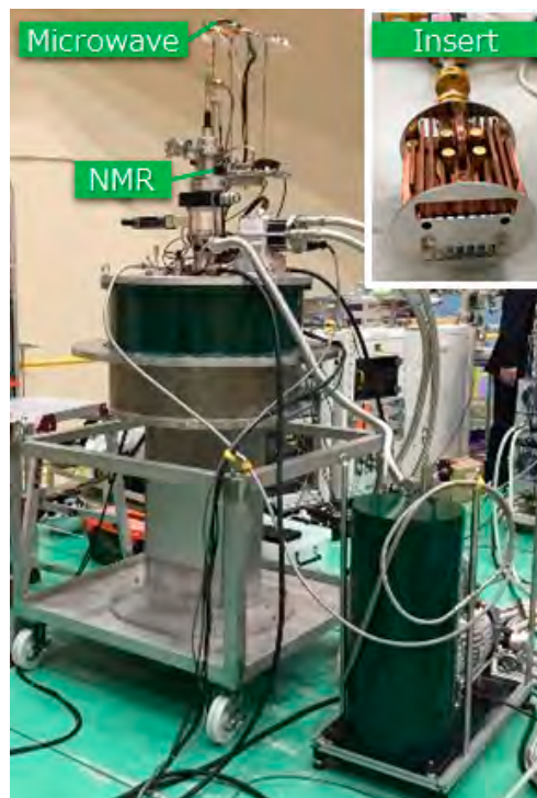
Figure 1. DNP apparatus for SCV-NR measurements using the cryogen-free transverse magnetic field magnet of BL15 [2, 3].
