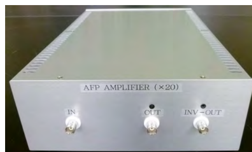
Figure 2. An RF amplifier developed for AFP NMR of ^3\text{He} NSF.
