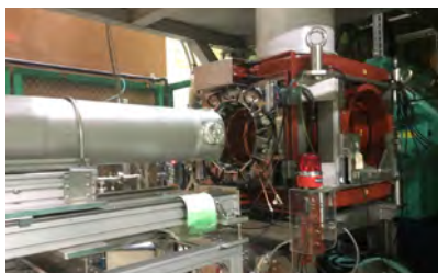
Figure 1. \mu SR spectrometer with the dilution refrigerator and the fly-past chamber at D1.
