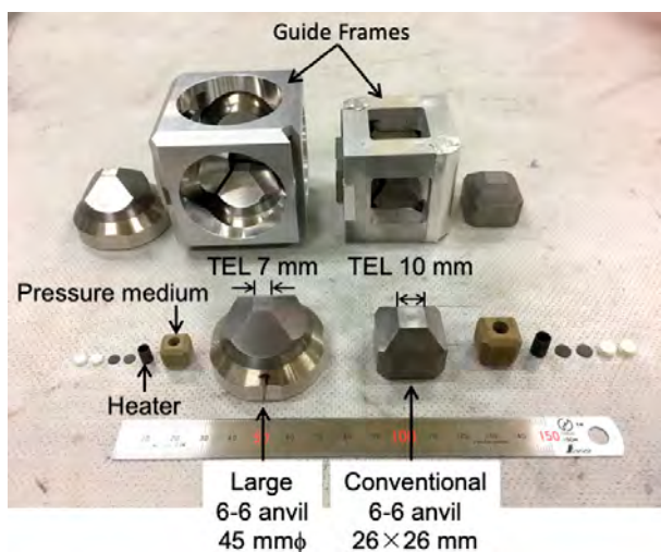
Figure 1. Conventional 6-6 anvils and large 6-6 anvils with shrink-fitted jackets. Guide frames and cell assemblies are also shown.
