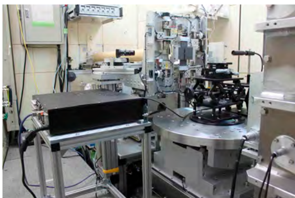
Figure 2. LED light source system with four modules with different peak energies used on SHARAKU (BL17)
