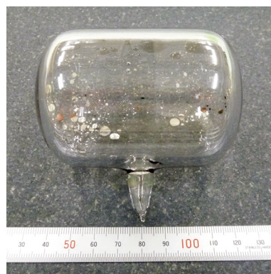
Figure 1. A cylindrical shape ^3\text{He} SEOP cell made of GE180 with ^3\text{He} gas of 3.4 atm and alkali metals inside. The shiny metallic spots are a mixture of rubidium and potassium.
