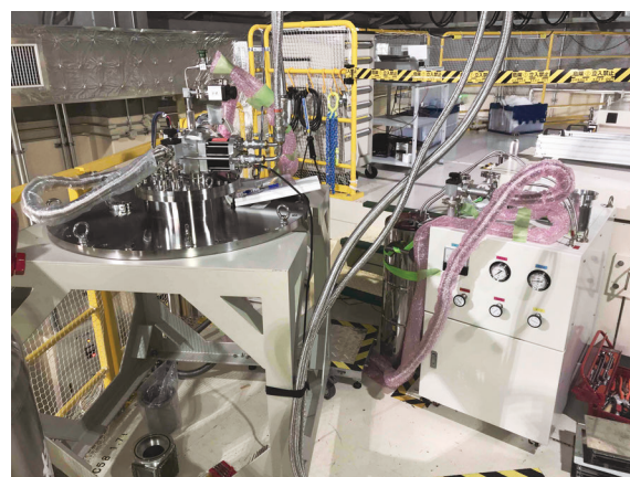
Figure 3. The 1K cryostat system during commissioning. A problem was found with the needle valve in the ^3\text{He} line, and repair is scheduled for FY2019.
