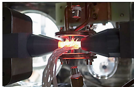
Figure 2. The sample area of a new sample environmental device for horizontal loading equipped with an induction heating system.
