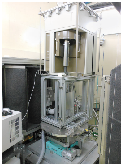
Figure 2. High precision gas/vapor adsorption measurement instrument installed on a sample stage of TAIKAN.
