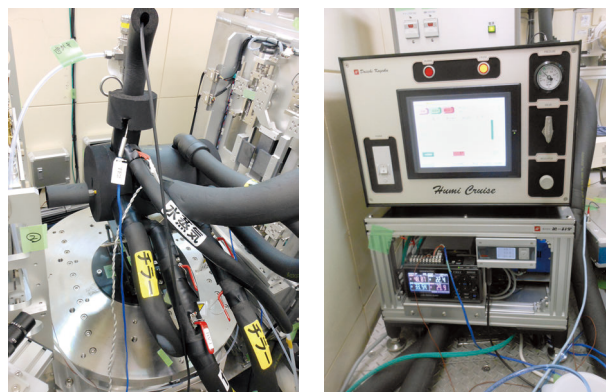
Figure 1. Photographs of the humidity-control system: sample chamber (left) and humidity generator (right).
