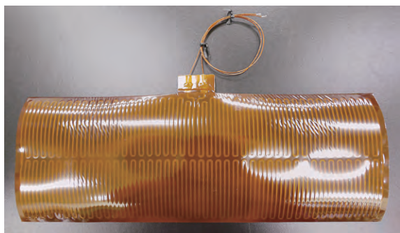
Figure 4. A prototype polyimide heater. This flexible heater is designed to wrap the cylindrical oven made of aluminum. The heating power is 270 W, and the maximum temperature is 300^\circ\text{C} .
