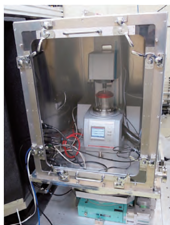
Figure 5. The rheometer and its box on the goniometer stage of BL15.
