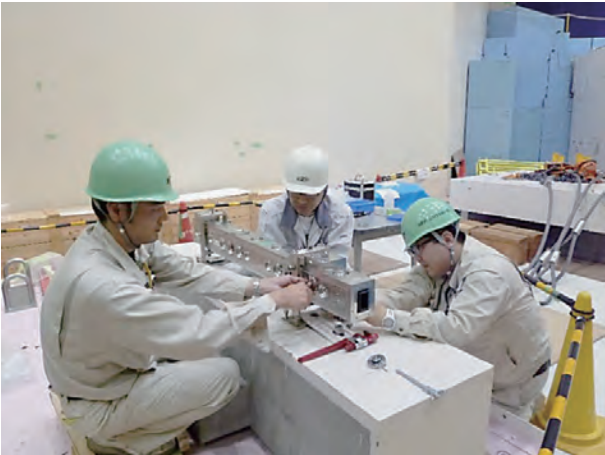
Figure 2. Replacement of supermirror of the final section of AMATERAS beam-transport.
