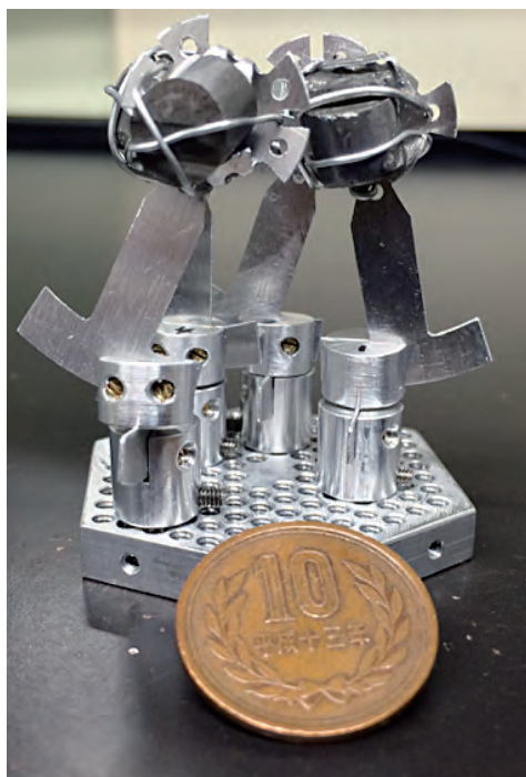
Figure 1. Co-aligned sample of \text{Mn}_3\text{Sn} (12 g). Alignment was performed using the forward scattering X-ray Laue apparatus in the Masuda Lab at ISSP.
