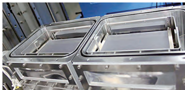
Figure 2. Photograph of the temperature-controlled stage for high temperature.
