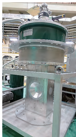
Figure 1. A 4 Tesla split-pair superconducting magnet.
