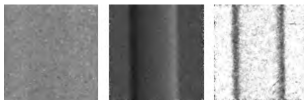
Figure 3. Resultant images of Talbot-Lau interferometry for aluminum rod. (Left) absorption-contrast imaging. (Middle) Differential-phase-contrast imaging. (Right) Visibility-contrast imaging.
