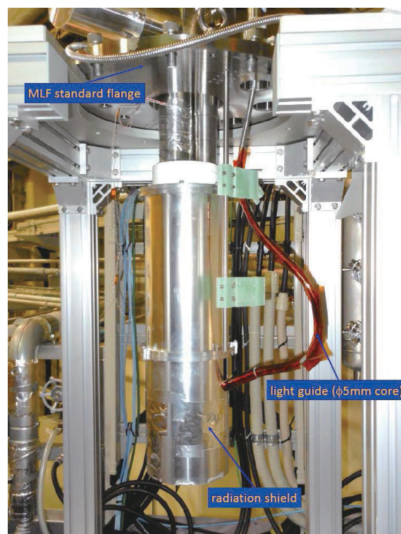
Figure 1. Side view of the cryostat for photo crystallography.
