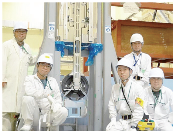
Figure 1. Installation of the muon rotating graphite target.
