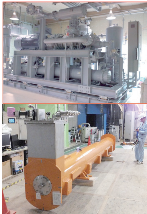
Figure 1. Photograph of the new compressor (above) and the solenoid (below).
