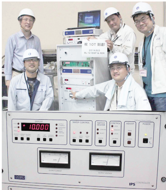
Figure 2. Successful operation of the superconducting magnet with the application of magnetic field of 10 T at the sample position of the HRC.
