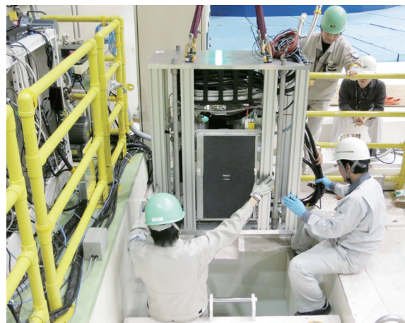
Figure 1. The Fermi chopper translation unit with the original and new Fermi choppers being installed on 4SEASONS by the technical support staffs.
