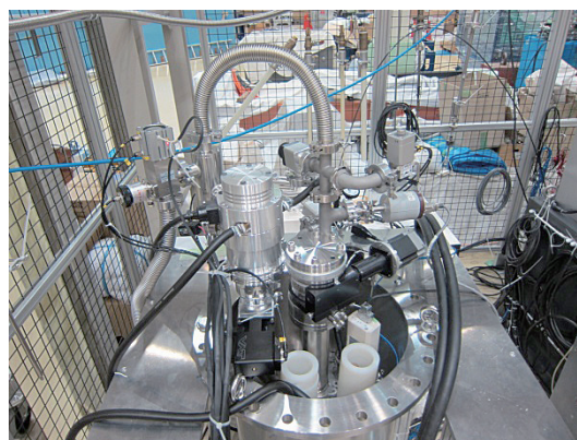
Figure 2. Improved vacuum pumping system of a high temperature furnace.
