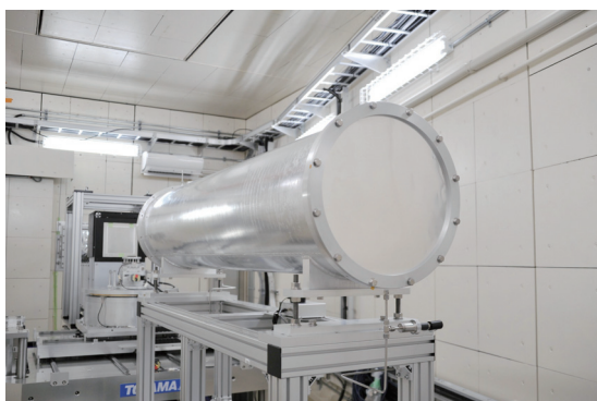
Figure 4. A flight tube (Front) and a detector (rear) in RADEN measuring room.
