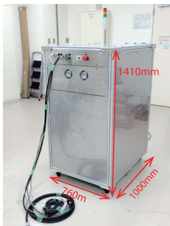
Figure 3. Photograph of the power supply.
