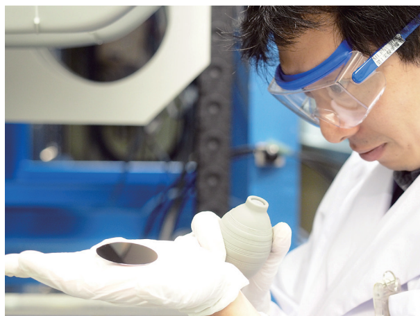
Norifumi Yamada checking a sample substrate for neutron reflectivity measurement at BL16 SOFIA.
