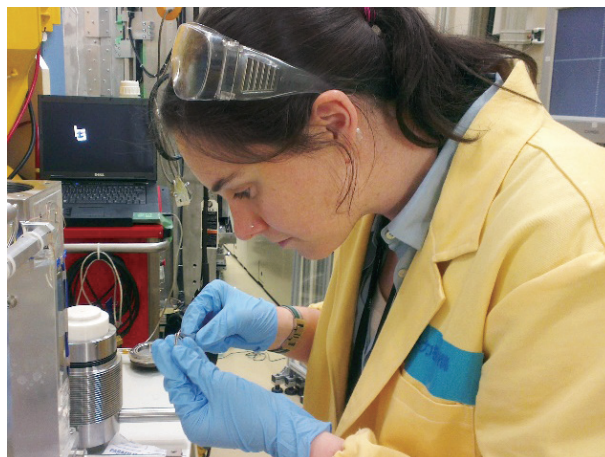
Maynard-Casely, Helen preparing the Mito cell for high-pressure neutron experiments at BL11.
