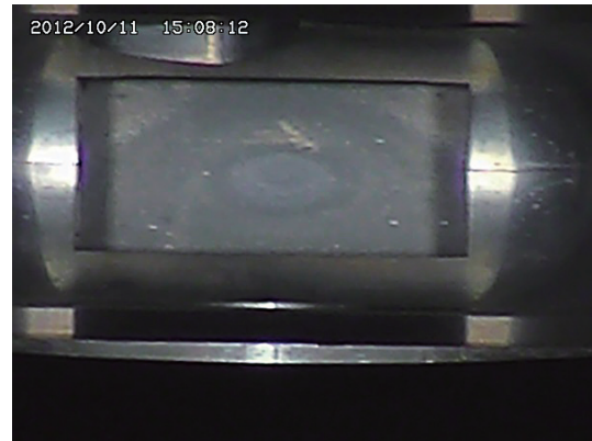
Figure 1. Surface of the 1 st PBW observed by high zoom WEB camera in October 2012.
