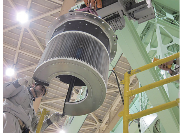
Figure 3. Radial collimator being installed on 4SEASONS by the technical support staffs.
