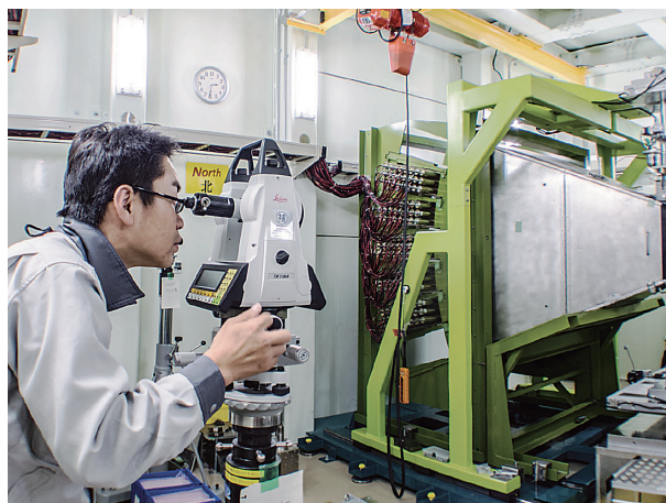
Takuro Kawasaki aligning a sample and optical devices at the Engineering Materials Diffractometer TAKUMI, BL19.
