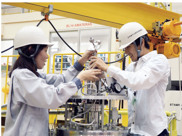
Seiko Kawamura (left) and Tatsuya Kikuchi (right) setting the sample stick into a top-loading cryostat at BL14.
