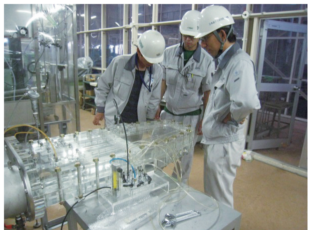
Katsuhiro Haga, Hidetaka Kinoshita, and Hideki Ueno discuss a water flow experiment on the new spallation neutron target.
