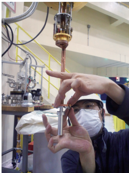
Keitaro Kuwahara (Ibaraki Univ.) loads a sample in the refrigerator at BL14.
