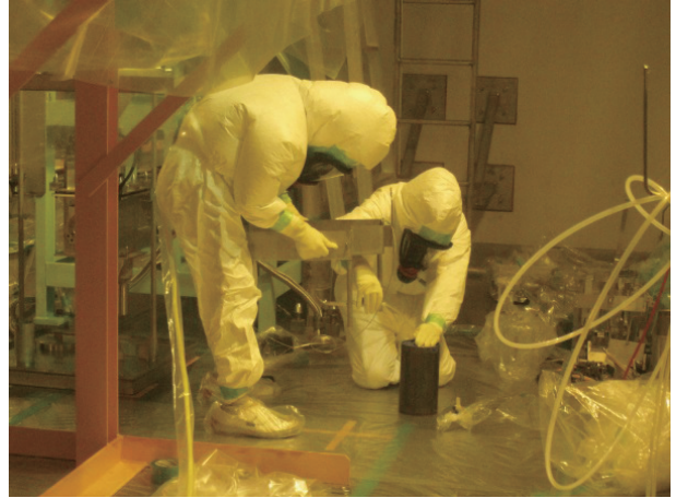
Members of the target group dressed in air-line suits and face masks carefully remove mercury from the target following an irradiation experiment in the hot cell.
