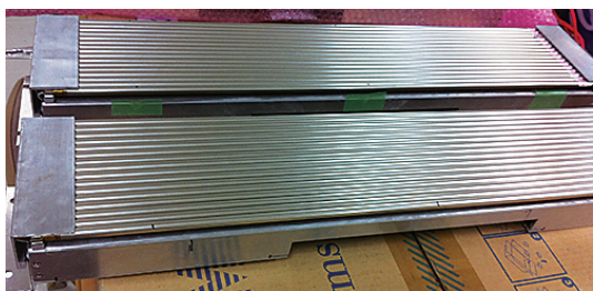
Figure 5. New position sensitive detector for SuperHRPD. The diameter is \phi 8 .
