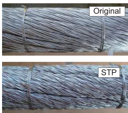
Figure 8. Photograph of the cable with original twisting pitch and STP.
