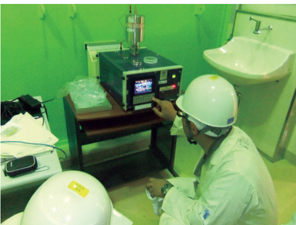
Measurement of tritium gas density during operation of the mercury target cover gas treatment system.
