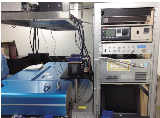
Figure 3. System of coherent Lyman- \alpha resonance radiation source at the muon U-line.
