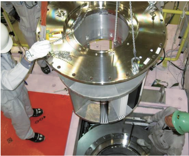
Figure 2. Test of a new oscillating radial collimator.
