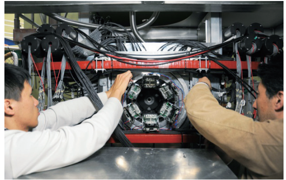
Masatoshi Hiraishi and Kenji M. Kojima work on the newly-installed 'Kalliope' detector system of the DOmega-1 spectrometer at the D1 experimental area.
