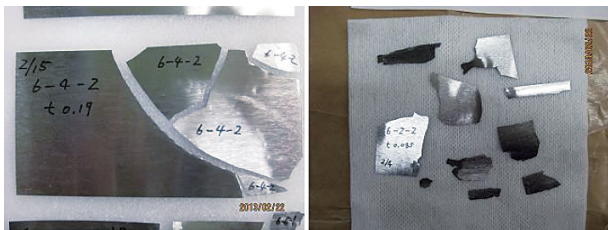
Figure 4. Pictures of the broken tungsten foils.
