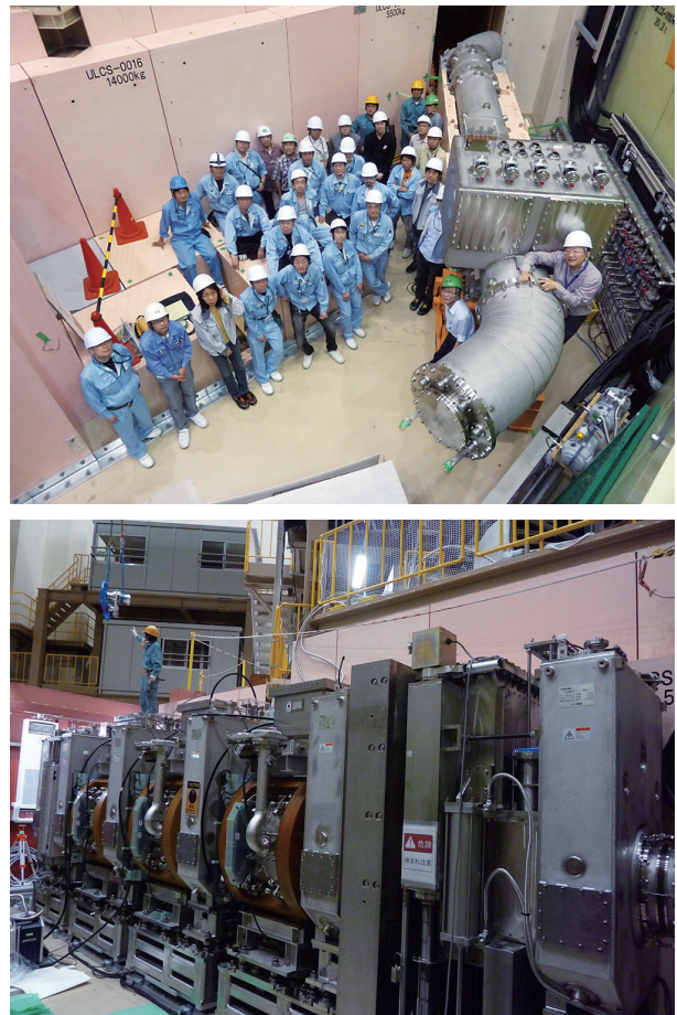
Figure 1. (Up), picture of the celebration of the delivery of the superconducting curved transport solenoid magnet. (Down), picture of the superconducting axial focusing magnets associated with three sets of \pm 400 kV DC separators.
