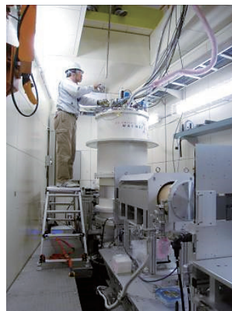
Figure 4. The 7 T superconducting magnet on the sample table of SHARAKU.
