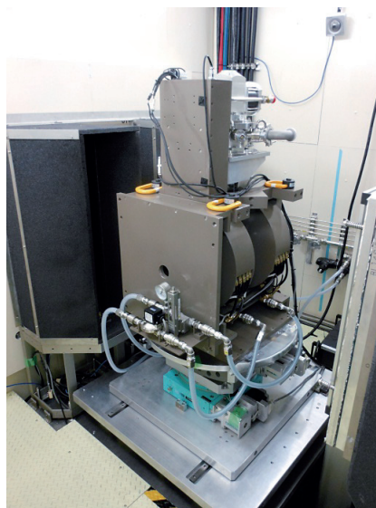
Figure 5. A 1Tesla-electromagnet with a 4K-cryostat.
