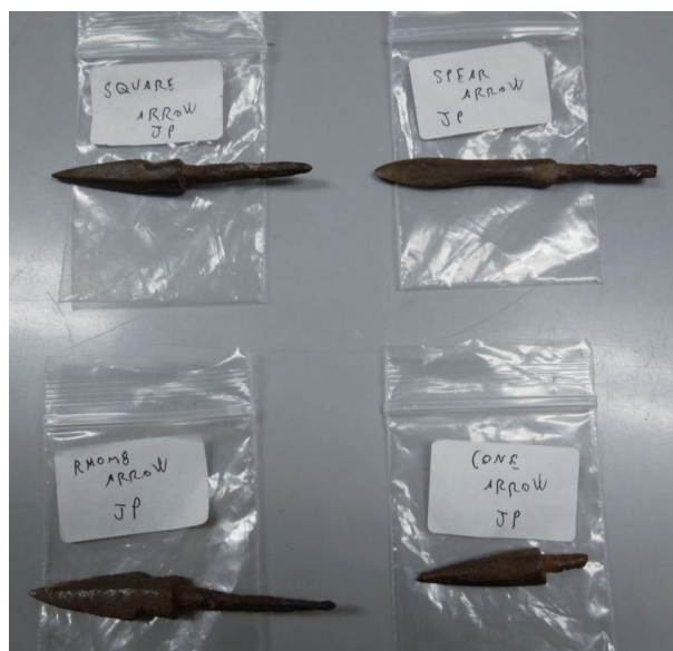
Figure 1. Picture of the four analyzed samples. Square (Sq) and rhomb (Rh) are low carbon steel, spear (Sp) is high carbon steel, and cone (Co) is iron.
