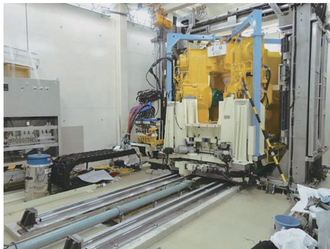
Figure 4. The 6-axis multi-anvil press “ATSUHIME” installed in the experimental hutch.
