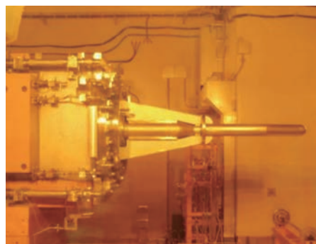
Figure 1. The first target vessel with plastically elongated seal bellows and the new replacement target vessel, which was redesigned to be compact and reduce the radioactive wastage.
