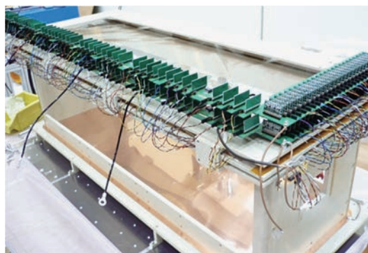
Figure 1. The time projection chamber for the precision neutron lifetime measurement at BL05.
