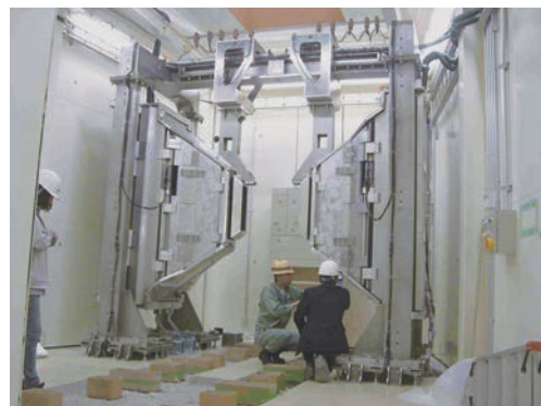
Figure 3. Detector banks with the foldable shielding panels and the alignment system for radial collimators.
