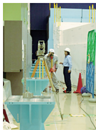
Figure 2. A survey of the neutron beam line on BL02. (July 28, 2010).
