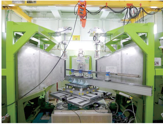
Figure 6. Off-line test at Takumi: 3.6 m long ITER- CS conductor.
