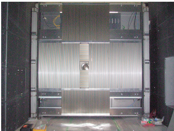
Figure 4. A small-angle detector bank with ^3\text{He} PSD tubes.
