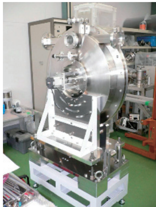
Figure 3. Doppler shifter installed at the unpolarized beam branch of the NOP beamline for the study of neutron optics and fundamental physics at the beam port BL05.
