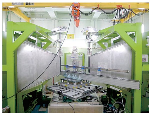
Figure 5. Off-line test using 3.6m long ITER- CS conductor.
