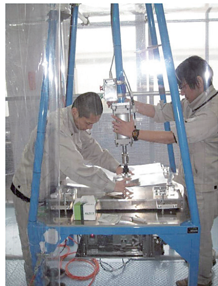
Figure 7. Procedure of gluing a Si wafer to the Al plate No.2.
