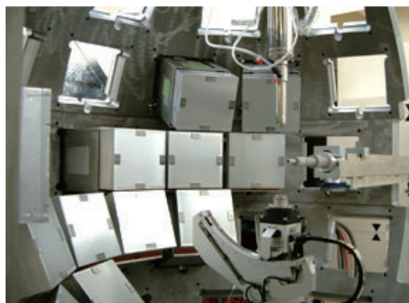
Photo. 2 A close-up view of the iBIX (14 detectors have been implemented in the instrument)
