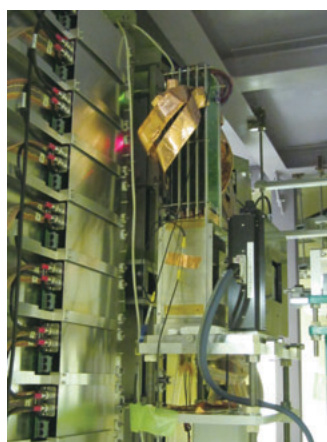
GEM detector system (left) used as neutron beam monitor, installed upstream of the NOVA diffractometer (right).
