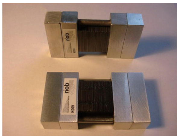
Fig.2 Pieces of prototype slit packages for the MAGIC chopper (collaboration with Th. Krist)
