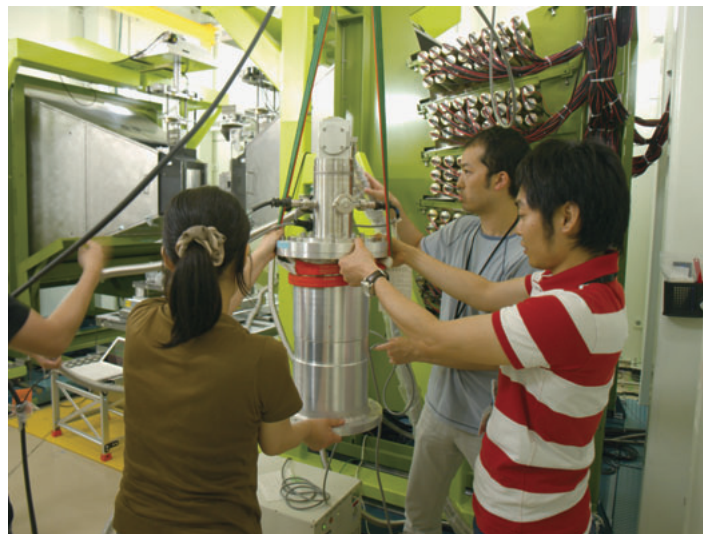
High-pressure group, Asami Sano (JAEA), Kazuki Komatsu and Masashi Arakawa (University of Tokyo), at TAKUMI (BL19) setting up the palm cubic-anvil cell installed in a cryostat to study structure of ice under high-pressure.
