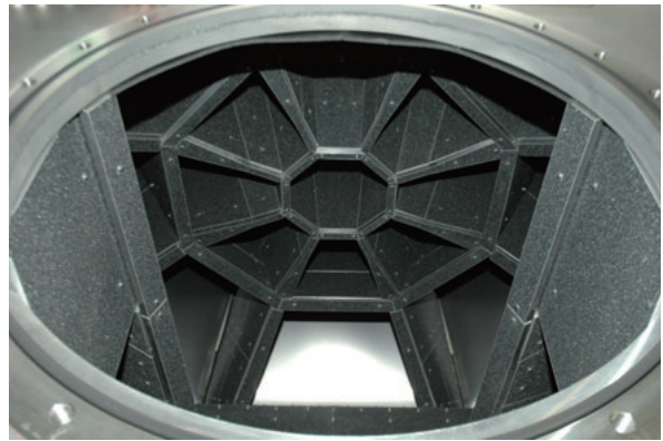
Fig.3 B_4C -resin tiles on the inner surface of the scattering chamber of NOVA diffractometer (BL21).
