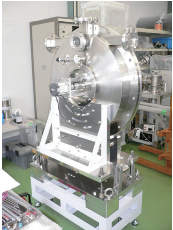
Fig.3 Doppler shifter installed at the unpolarized beam branch of the NOP beamline for the study of neutron optics and fundamental physics at the beam port BL05. A moving multilayer mirror of m=10 is installed to convert very cold neutrons ( v \sim 140 \text{ m/s} ) to ultracold neutrons by the Doppler shift.
