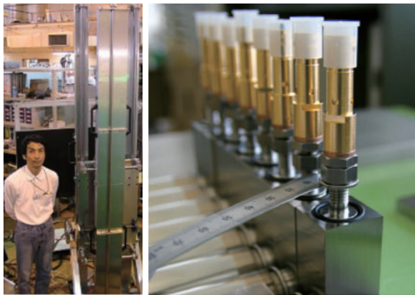
Fig.2 A 2.5m length PSD on the testing stand at the test port (left). A newly designed vacuum coupling end SKYN 2 (right)
