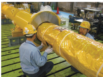
Fig.1 80K shield installing with thermal insulators.
