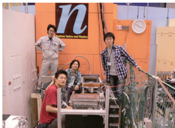
Fig. 2 Installation of a spin flip chopper for the measurement of neutron lifetime at the polarized beam branch of the NOP beamline.
