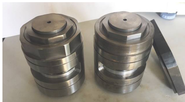
Figure 2. (Left) A modified load clamp and (right) an original load clamp with a jig to grab it with a handle bar. The screw to hold the load clamp is changed into a hexagon nut.
