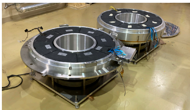
Figure 3. Detector units (top and bottom) installed in the vacuum scattering chamber. Various colors of cables, such as LAN-cable, signal cables, and power cables, are connected to the units.
