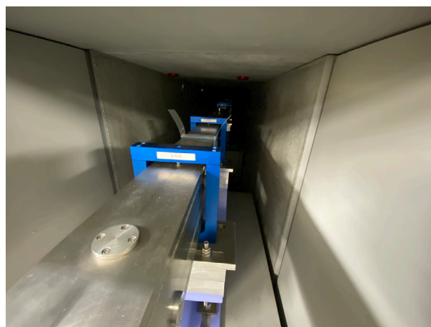
Figure 4. Partial view of the supermirror guide facing toward the decoupled poisoned moderator.
