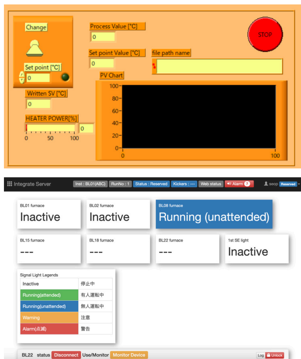
Figure 3. (a) Recording and control screens in LabVIEW. (b) Monitoring screen in IROHA2. The blue display indicates that the BL08 is in unmanned operation.
