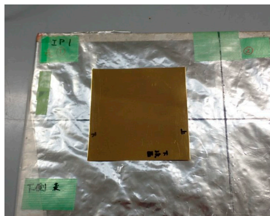
Figure 3. Picture of an imaging plate and the irradiated gold-foil for gamma-ray transfer.
