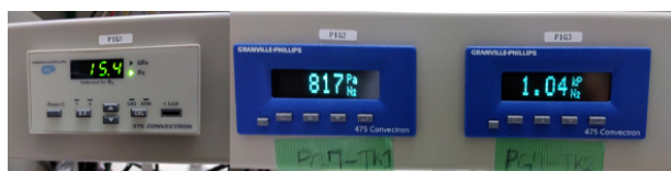
Figure 1. The vacuum gauge controller installed in the control room of 3NBT downstream. (Left: for inter-midterm exhaust, middle: for TK1, right: for TK2)
