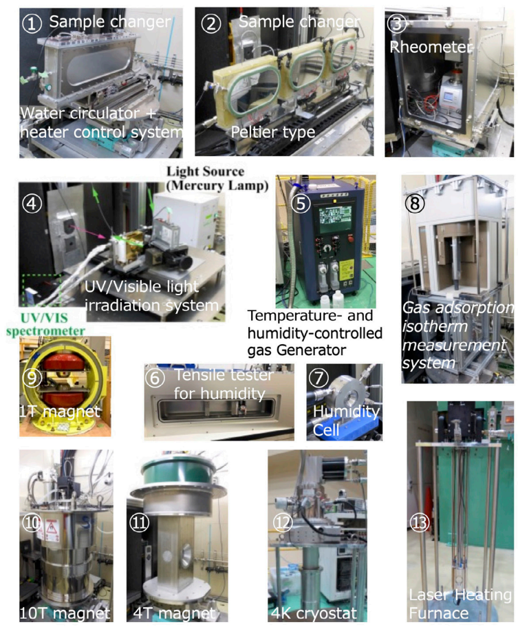
Figure 2. Sample environment devices developed at BL15 TAIKAN.
