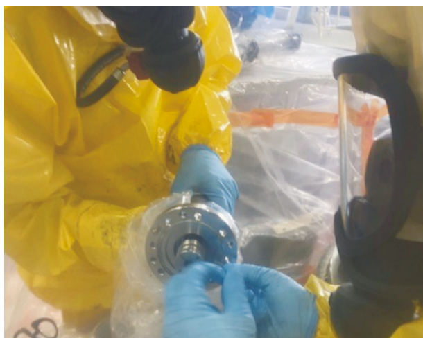
Figure 1. Rotary feedthrough exchanging working with airline mask and anorak suit.
