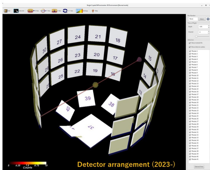
Figure 1. Detector arrangement of SENJU including the new area detector (No. 37).
