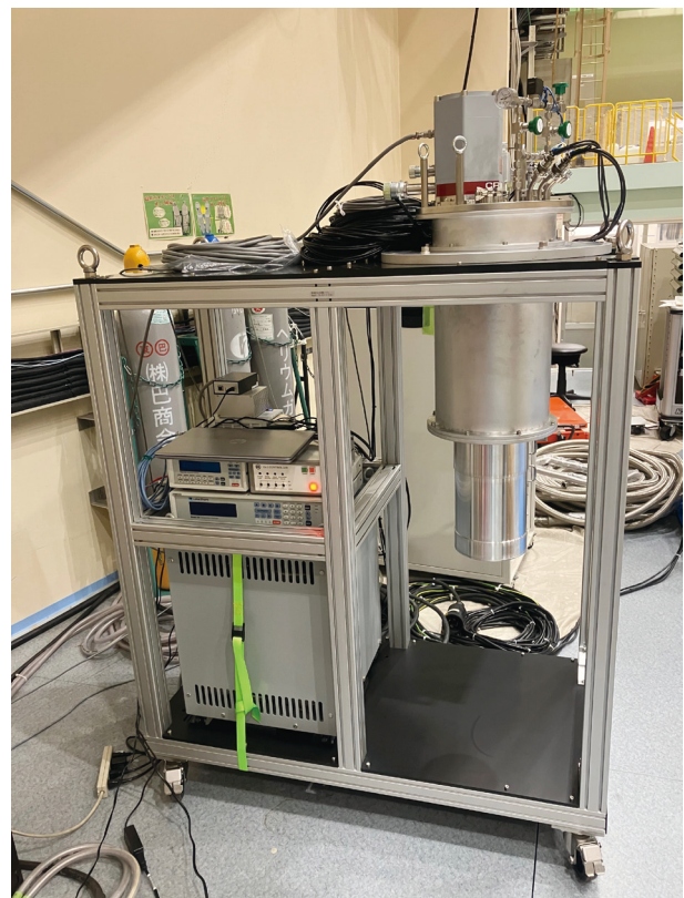
Figure 1. ^3\text{He} gas sorption type refrigerator delivered to the HRC in March 2023.
