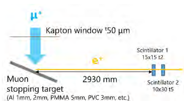
Figure 1. Setup of the beam intensity measurement.
