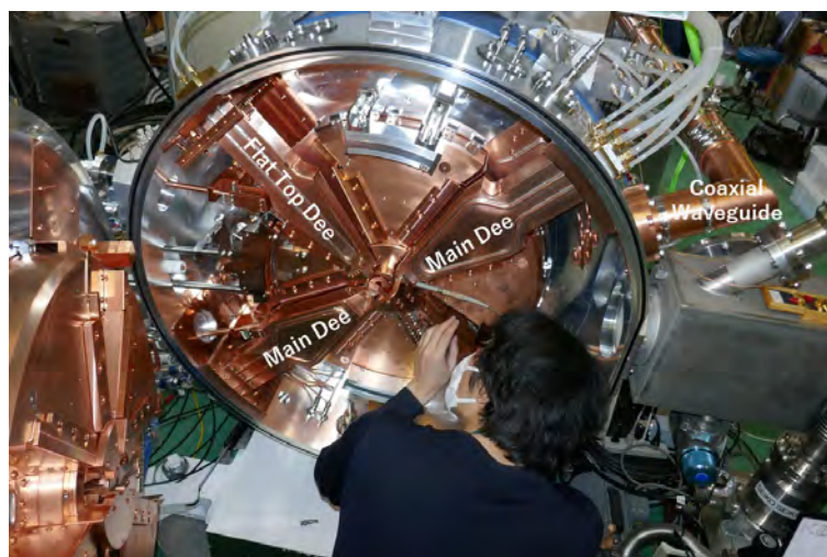
Figure 2. Internal structure of the 5 MeV muon-cyclotron. The ultraslow muon beam is injected at the center, and is accelerated by the Dees. The RF power is provided by the coaxial waveguide.
