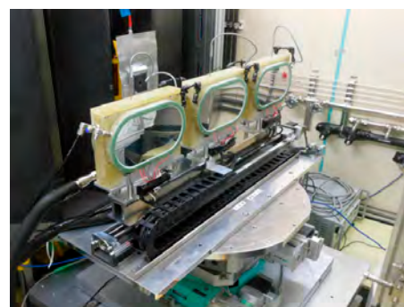
Figure 2. A Peltier-type sample exchanger.
