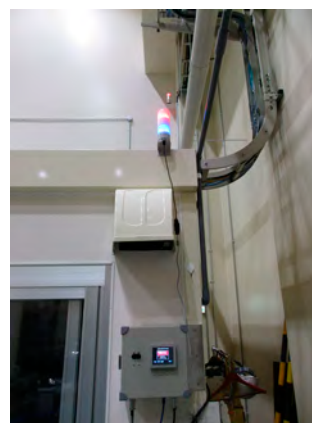
Figure 4. Remote monitoring system, used for high temperature experiment on SENJU.
