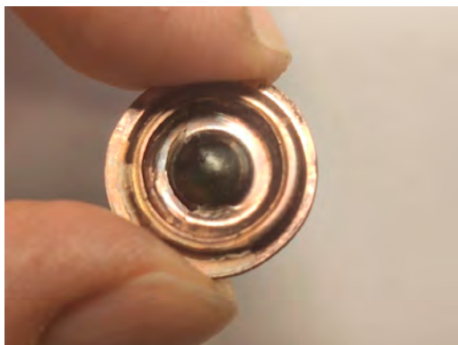
Figure 2. Picture of a sample (black sphere inside the metallic gasket) after compression of \text{CS}_2 to 8 GPa and subsequent pressure release.
