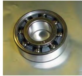
Figure 3. Solid-lubricant bearing used in the MLF J-PARC.
