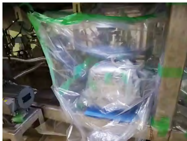
Figure 2. Photo of the vacuum pump in the barrier box before the replacement.
