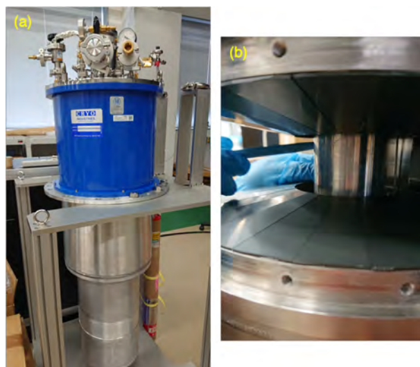
Figure 1. Photographs of the superconducting magnet suitable for BL02. (a) whole view, (b) coils of magnet covered by \text{B}_4\text{C} tiles.
