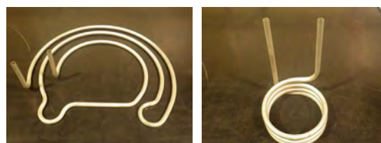
Figure 2. Test pieces of cooling water pipes to be buried in the target assembly.
