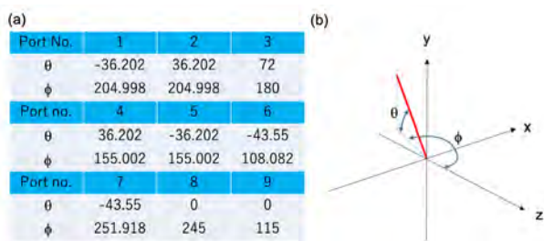
Figure 3. (a) Angles at each port in the Hemispheric chamber. (b) When the direction of the beam (from upstream to down-stream) is defined as z-axis, \phi and \theta are an angle from the z-axis in the horizontal plane (xy plane) and an elevation angle from vertical axis (y).
